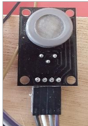
Fig. 13. MQ-7 carbon monoxide detector.
