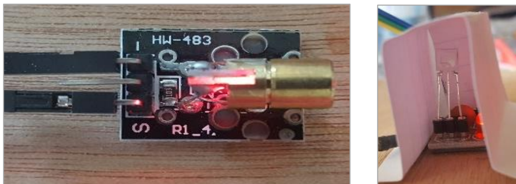
Fig. 15. Laser transmitter and diode detector.
