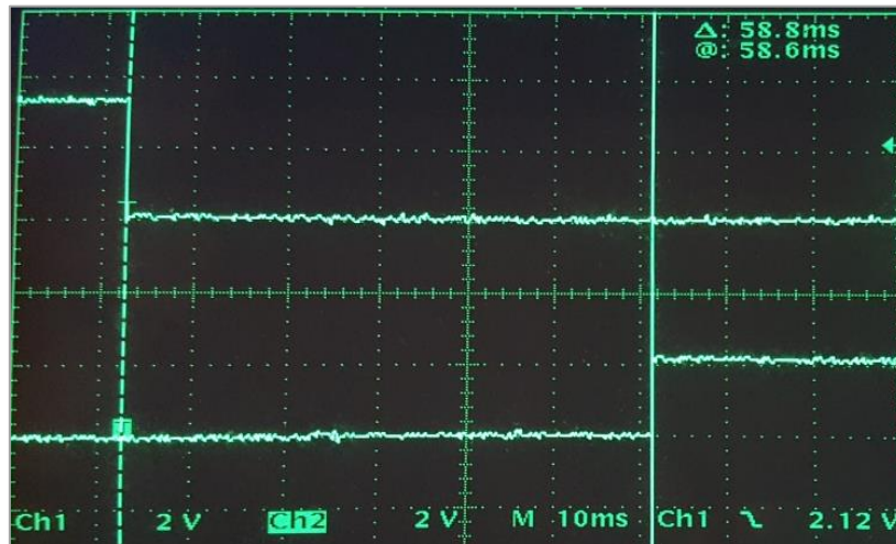
Fig. 23. Button press (Top) and door relay (Bottom).
